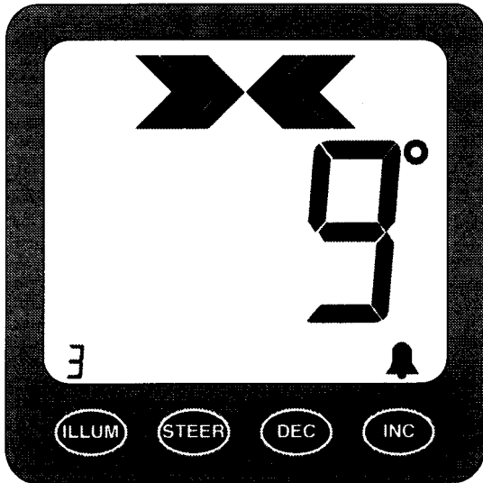
FIGURE 6 - Alarm Boundaries set at +/- 9°
